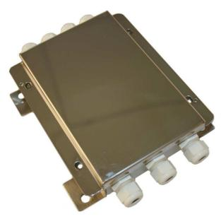
Stainless steel junction box with IP65 protection from water and dust, and fitted with electronic board for junction and equalisation of four or six load cells. Terminal board with screws for easy connection of the load cells and signal adjustment trimmers for accurate and reliable equalisation.
