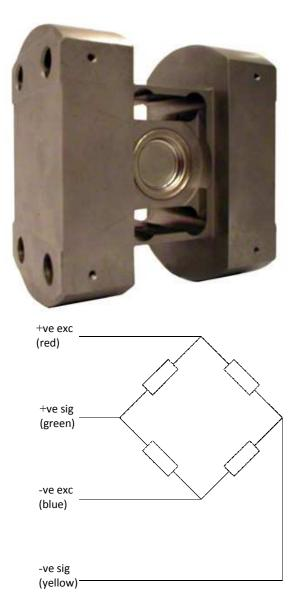
The Bin Lift Cell range of load cells are approved for commercial weighing to **OIML R60 2000**. The side mounting load cell has been specifically designed for the extremely high fatigue stress and impact loads experienced in onboard vehicle weighing. The fully welded construction of the Bin Lift cell makes it an ideal unit for the hostile environment experienced in applications where durability and high accuracy are of paramount importance.
